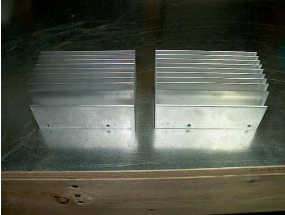
51. This is the cut heat sink after cleaning off the cutting oil and metal debris.
