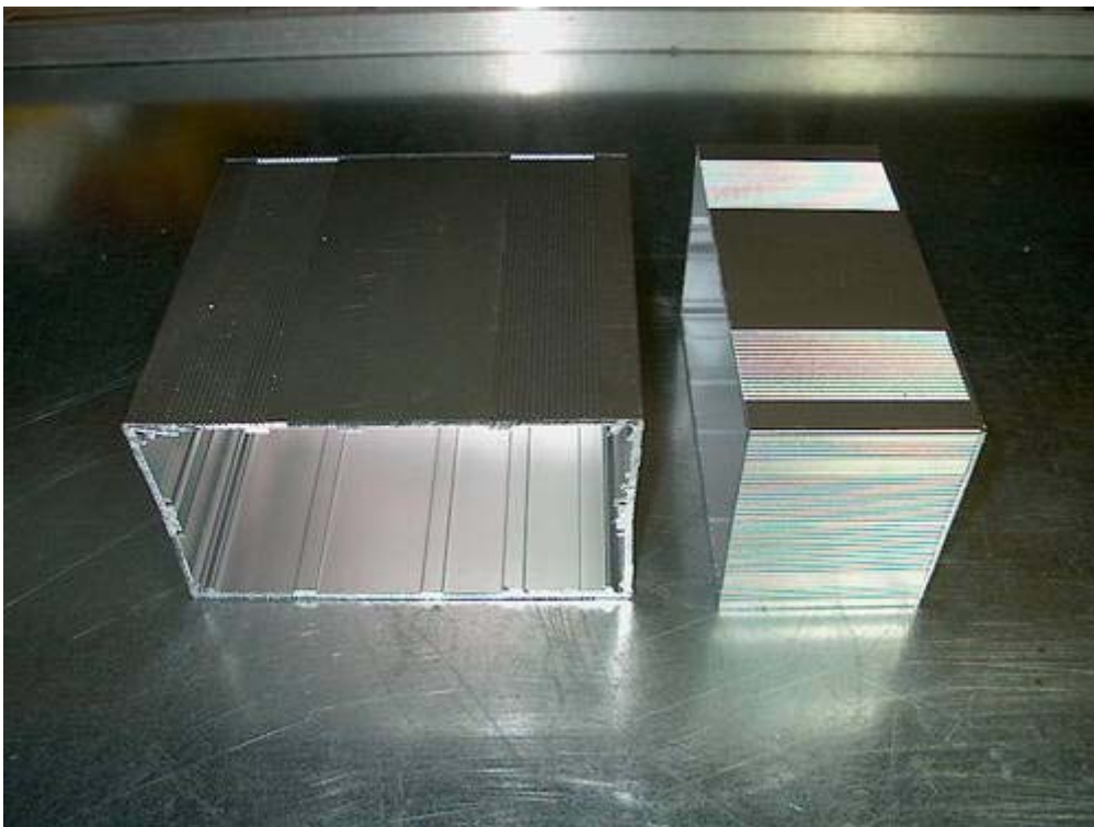
51. This is the cut heat sink after cleaning off the cutting oil and metal debris.
