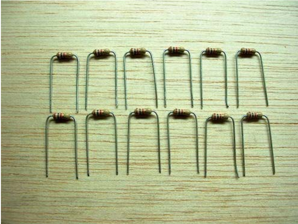
24. Here is an army of 1k 1/4 watt resistors with the leads formed to go into positions R1, R2, R3, R7, R8, R9, R10, R13, R16, R21, R22, and R23.
